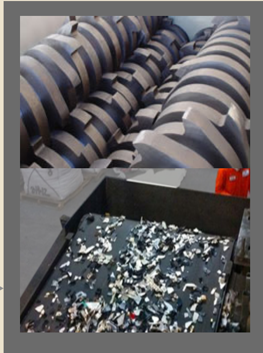
Shredding and automated sorting
